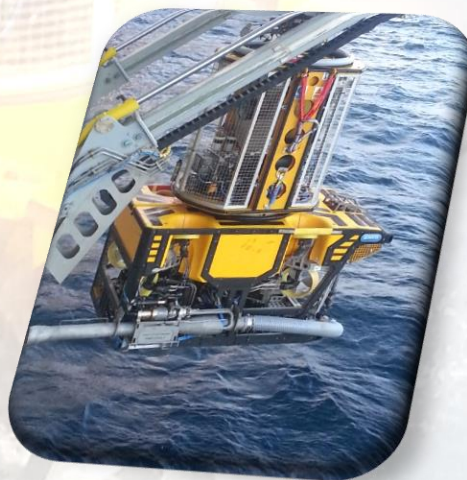
Picture to the right shows a Predator MKI T-8 mounted to SMD Quantum ROV
